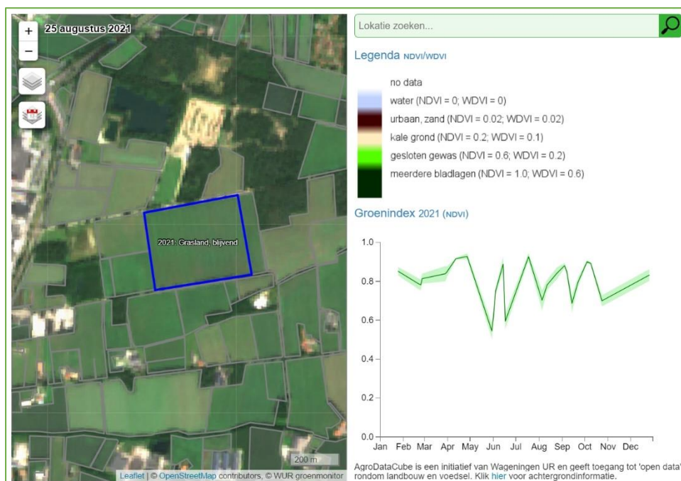
Figure 14: Screenshot of the green Monitor, where the graph highlights 5 mowing cuts as sharp dips in the NDVI curve of the selected grassland parcel
